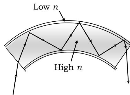
Optical cable consists of a number of glass or quartz fibres. Each fibre consists of a core and a cladding. The refractive index of the core is higher than that of the cladding. Light entering into the core satisfies the two conditions for total internal reflection. Hence it undergoes repeated total internal reflections along the fibre and finally comes out with negligible energy loss.
